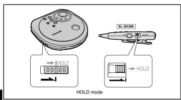
This function causes the unit to ignore short, accidental button presses. (The disc lid can still be opened and closed.)
